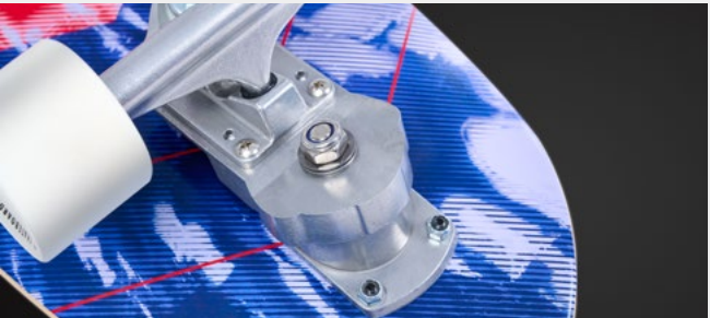
ATOMIC TRUCK The ATOMIC truck system is a responsive, sharp turning and surf carving machine. Built with a spring-loaded surfskate truck, it works by a spring inside it and by compression. It is perfect for riders to practice surf maneuvers such as bottom turns or cutbacks.
