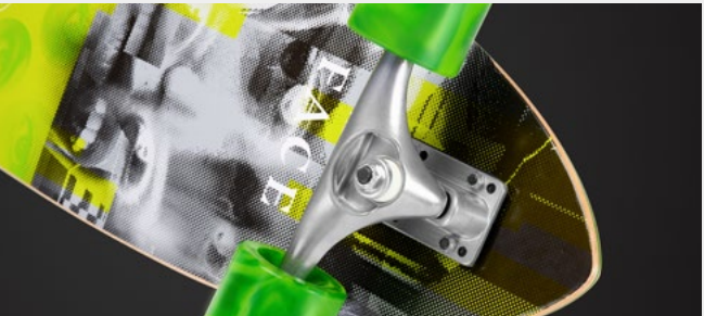
SX 4.0 TRUCK The SX 4.0 truck features a set of spherical wave cams that translate axle rotation into increased force by compressing a solid compression spring. It allows for tight turns and incredible speed when cruising.
